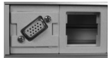
Figure 5: VGA coupler orientation
