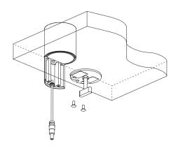
Beneath work surface, slide cord protector back into slot of clamp bottom plate.
