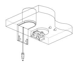
Then reinstall (2) bottom screws to reassemble clamp bottom plate to upper clamp.
