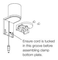
Fit upper clamp in desired location on work surface.
