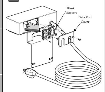
2 Install Data Port Options (VGA, RJ45, HDMI, BLANK)
