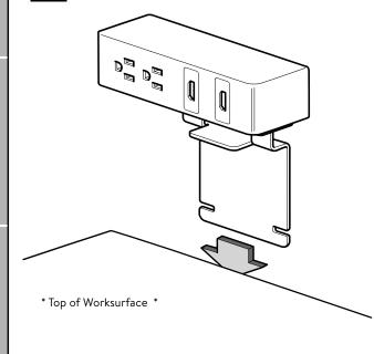
Install Bottom Bracket Under the Worksurface
