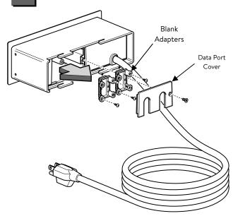
Install Data Port Options (VGA, RJ45, HDMI, BLANK)
