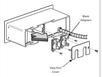
Install Data Port Options (VGA, RJ45, HDMI, BLANK)
