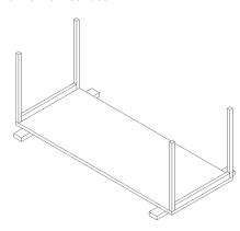
2. Apply weight plates to the center of the worksurface or stand directly on the work surface to create a counter bow in the work surface. Maintain the counter bow through Step 4.
