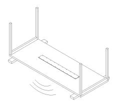
CRITICAL: 3/16" holes must be predrilled before screws are installed.
