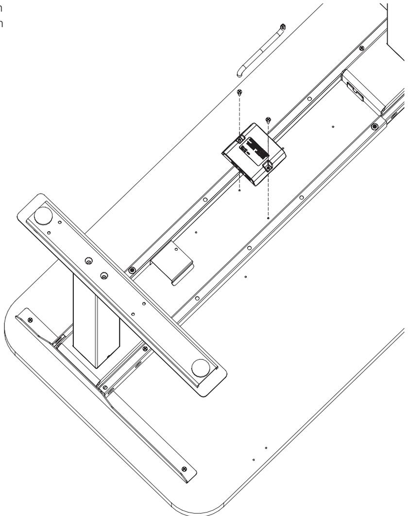
18. Connect the legs to the control box first, then connect the handset to the control box. It does not matter which port you use, just be sure the connections are secure. Next, connect the power cord to power supply but do not plug the cord into the wall until instructed to do so. Slide the power supply into the holder. Then connect the power supply to the control box.
