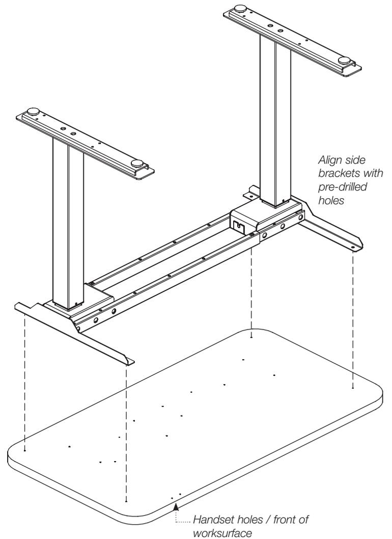
12. When in position, lift the frame just enough to slide the power supply holder under the crossbars but do not install the power supply yet. Ensure the holder starts about 2" from the motor housing.
