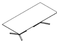
Rectilinear (Square or Curved Corners) D: 48, 54, 60" W: 96, 108, 120" H: 29"
