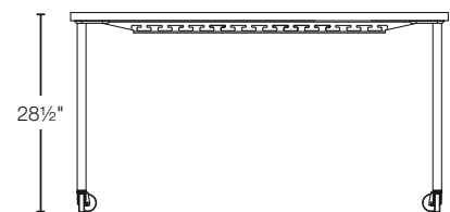
Side Elevation of Desk Height, with Casters
