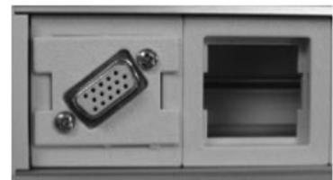
**Figure 5: VGA coupler orientation**
